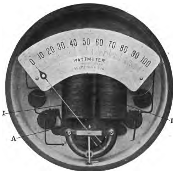
FIG. 3.—General view of Dr. Sumpner's Wattmeter.
